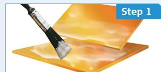
Ensure that the components are clean and free of oil etc. Make the flux into a creamy paste using water and apply to the joint area.
