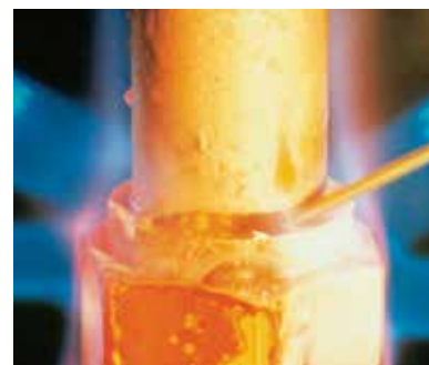
Flux protects the component from oxidation as the brazing filler metal flows
